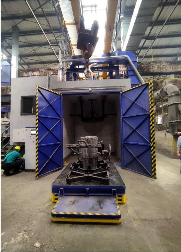
Fig. 3 The closed walled variant of the modification cabin for ladles up to 6t (part of the equipment is an automatically moving modification vehicle with a load capacity of 10t and electrically controlled wing doors)
