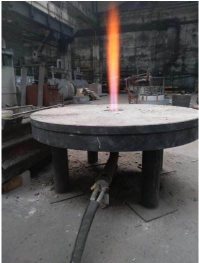
Fig. 7 Heating jigs of the ladles
