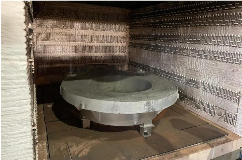
Fig. 6 Sintering of the lining of the modification cabin cover
