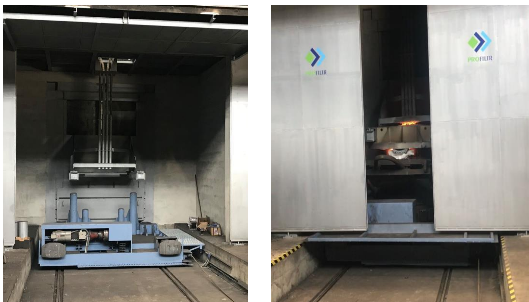
Fig. 2 The closed walled variant of the modification cabin for ladles up to 30t
