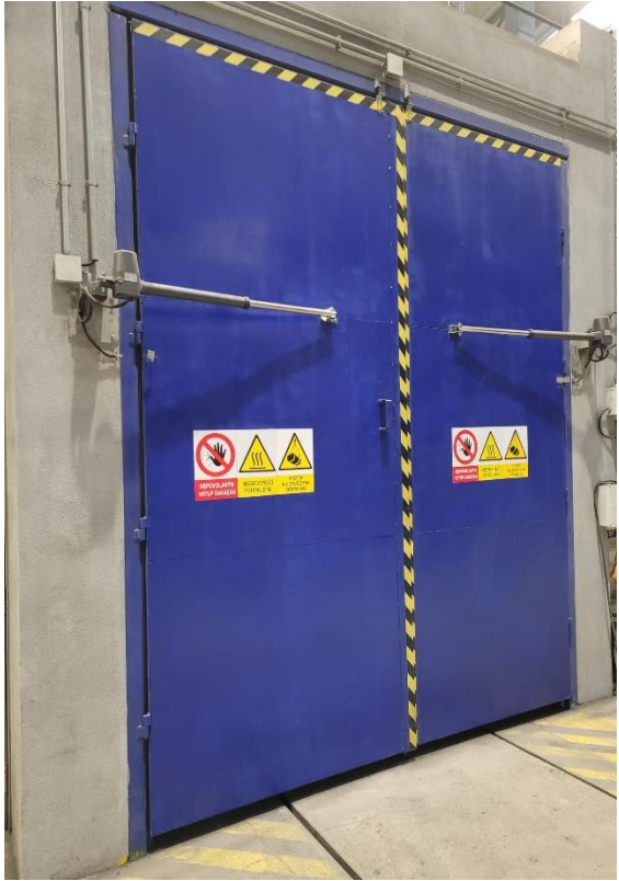
Fig. 3 The closed walled variant of the modification cabin for ladles up to 6t (part of the equipment is an automatically moving modification vehicle with a load capacity of 10t and electrically controlled wing doors)
