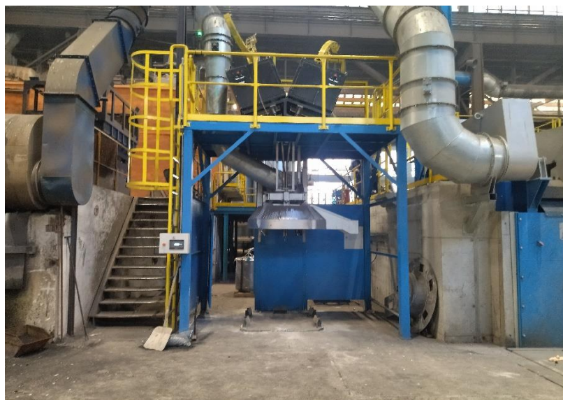
Fig. 4 The open variant of the modification cabin for ladles up to 6t
