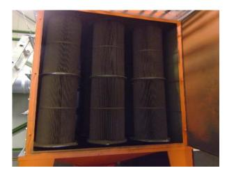
Delivery and replacement of cartridge filters, also for the extraction equipment of our competitors.
